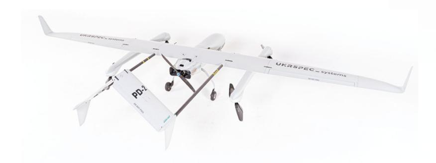
PD-2 is a multipurpose modular fixed-wing UAS with a wide range of options and payloads to fit any mission and operational environment. PD-2 is a conceptually new product obtained through a large list of innovations and upgrades based on the long-term operation history (more than 10,000 flight hours) of the previous flagship UAS PD-1
