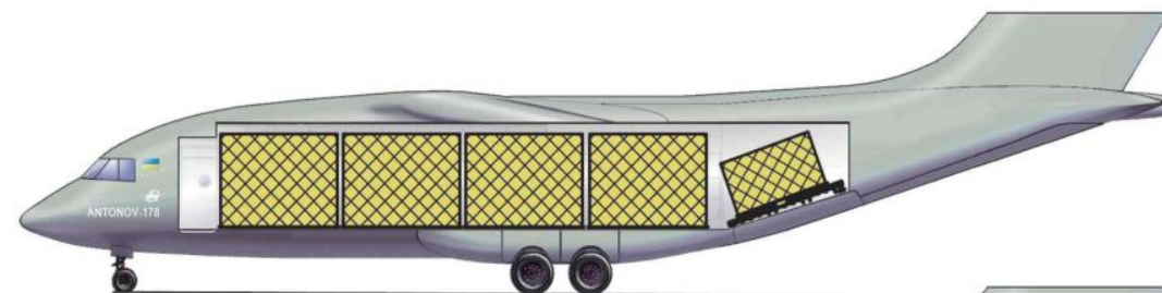
Four 88x125 inch and 88x108 inch pallets on cargo ramp
