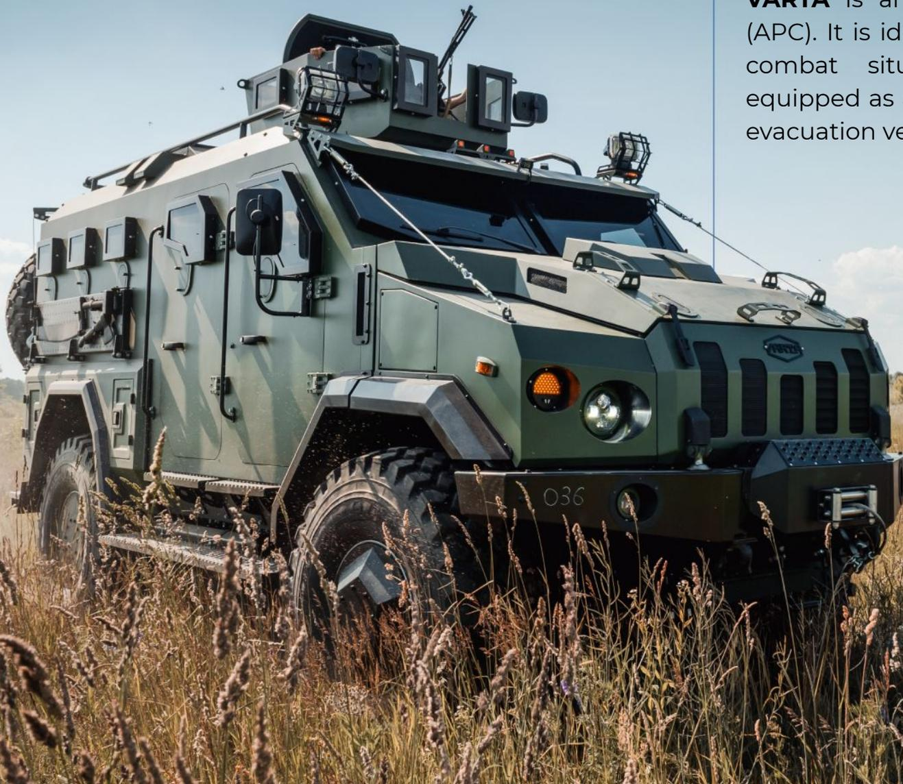
The vehicle compartment is made from specialized 560 steel grade which protects crew from armored piercing incendiary ammo up to 7.62mm. VARTA uses a V-shape hull structure to accommodate anti-mine seats, giving crew members protection to withstand detonation of charges up to 6 kg of TNT. VARTA includes a fighting module equipped with either 7.62 mm or 12.7 mm machine gun. The vehicle has 10 gun ports around with the feasibility of accommodating a UBGL (Under-Barrel Grenade Launcher)
